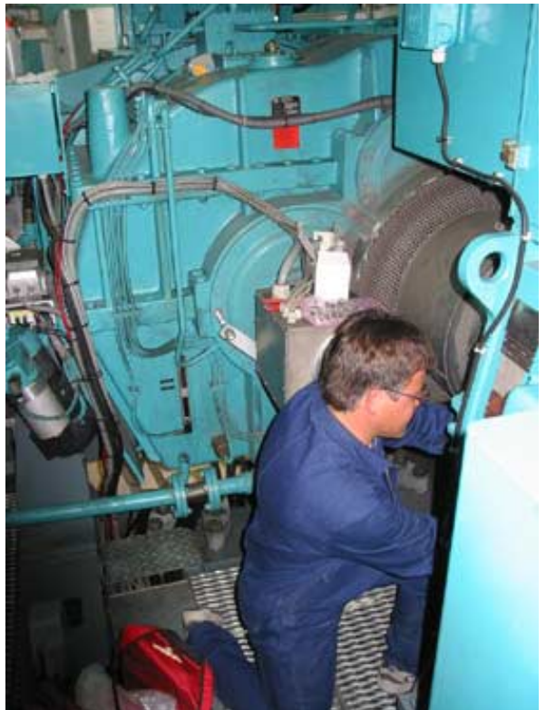
Dr. Becker (Flender Service) and R. Schühle (PRÜFTECHNIK Condition Monitoring) commissioning a monitoring system on a 1.5 MW wind turbine.
