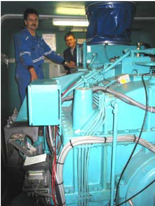
Dr. Becker (Flender Service) and R. Schühle (PRÜFTECHNIK Condition Monitoring) commissioning a monitoring system on a 1.5 MW wind turbine.
