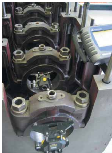
Fig.1: Laser equipment for monitoring the bearing saddles
