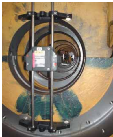
Fig.3: The laser transmitter with magnetic mounts
